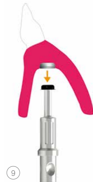
9 Removal of the processing plug-in part
