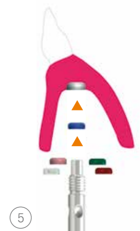
5 Insertion of the definitive matrix
