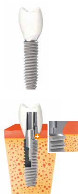
Integrated platform switching in the case of the BoneTrust® plus hex and cone implants
