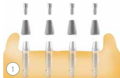
1 Screw the titanium bar base onto the BoneTrust® one laboratory analogue in the working model
